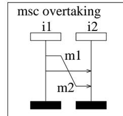
FIGURE 2. Basic Message Sequence Chart with overtaking
