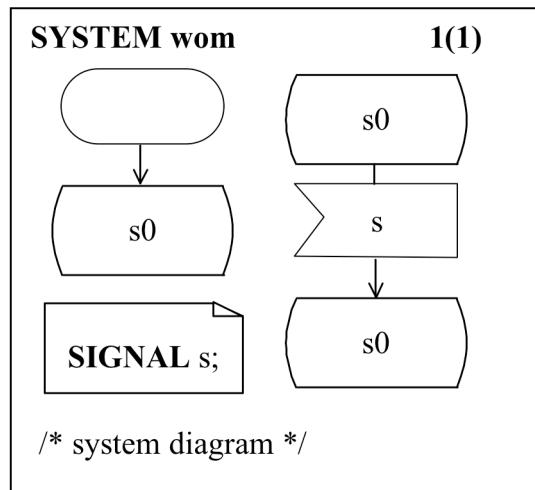
This is the system diagram for the previous example in Basic SDL-2010.
